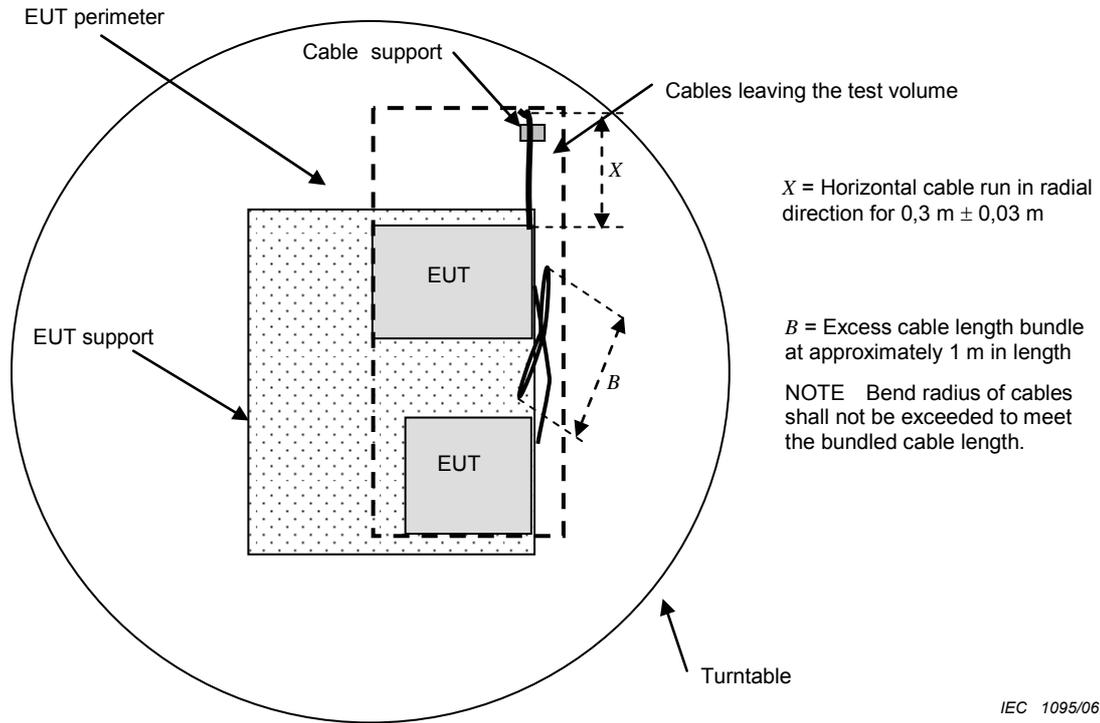
Figure 12 – Test set-up for floor-standing equipment, Top view
