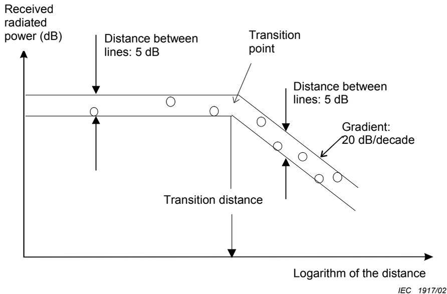
**Figure 17 – Determination of the transition distance**
