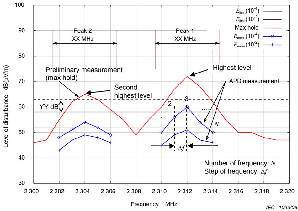
Figure E.1 – Example of APD measurement method 1 for fluctuating disturbances
