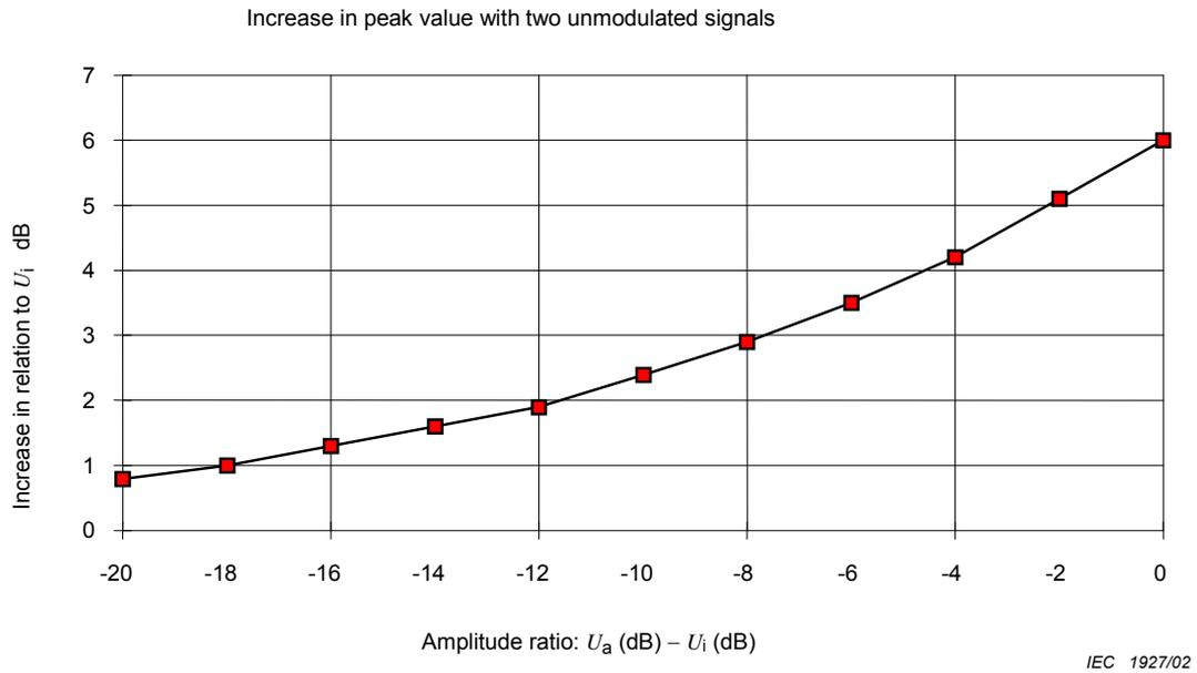
**Figure A.10 – Increase of peak value with superposition of two unmodulated signals**
