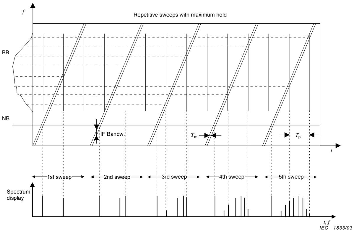
$T_p$  is the pulse-repetition interval of the impulsive signal. A pulse occurs at each vertical line of the spectrum-vs.-time display (upper part of the figure).
