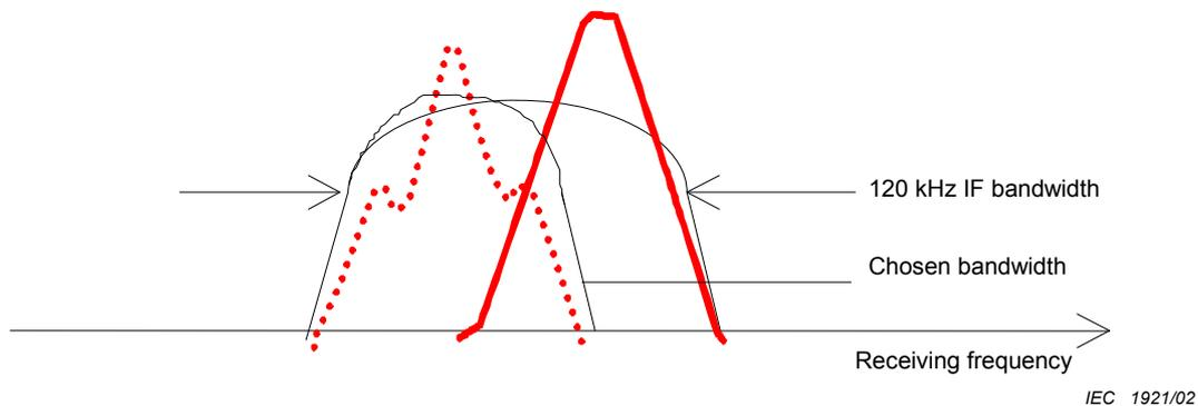
**Figure A.4 – Disturbance by an amplitude-modulated signal (dotted line)**
