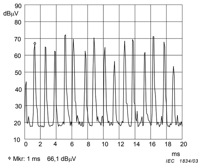
Disturbance from a DC collector motor: due to the number of collector segments the pulse repetition frequency is high (approx. 800 Hz) and the pulse amplitude varies strongly. Therefore for this example, the recommended measurement (dwell) time with the peak detector is > 10 ms.
