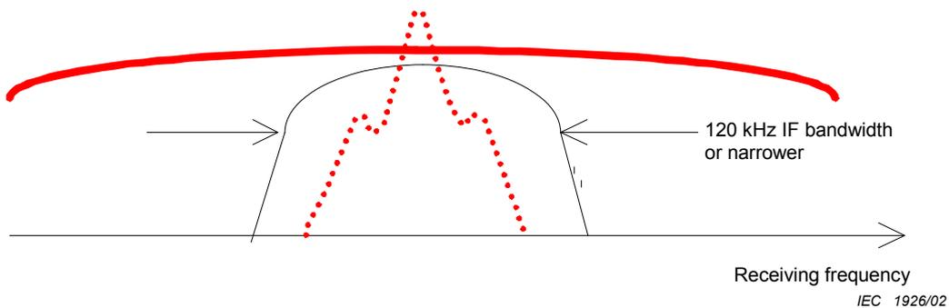
**Figure A.9 – Amplitude-modulated EUT disturbance (dotted line)**
