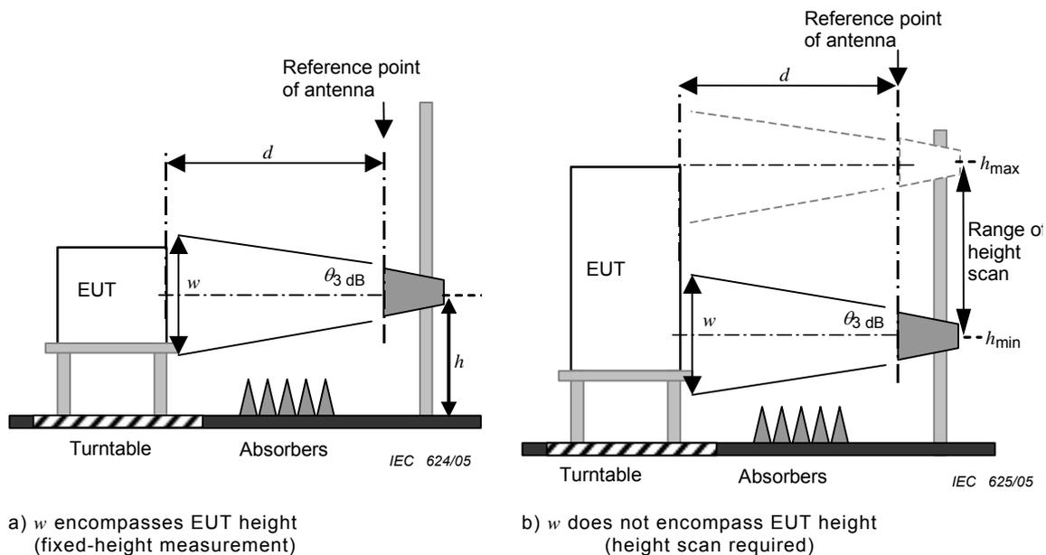
**Figure 13 – Illustration of height scan requirements for two different categories of EUTs**
