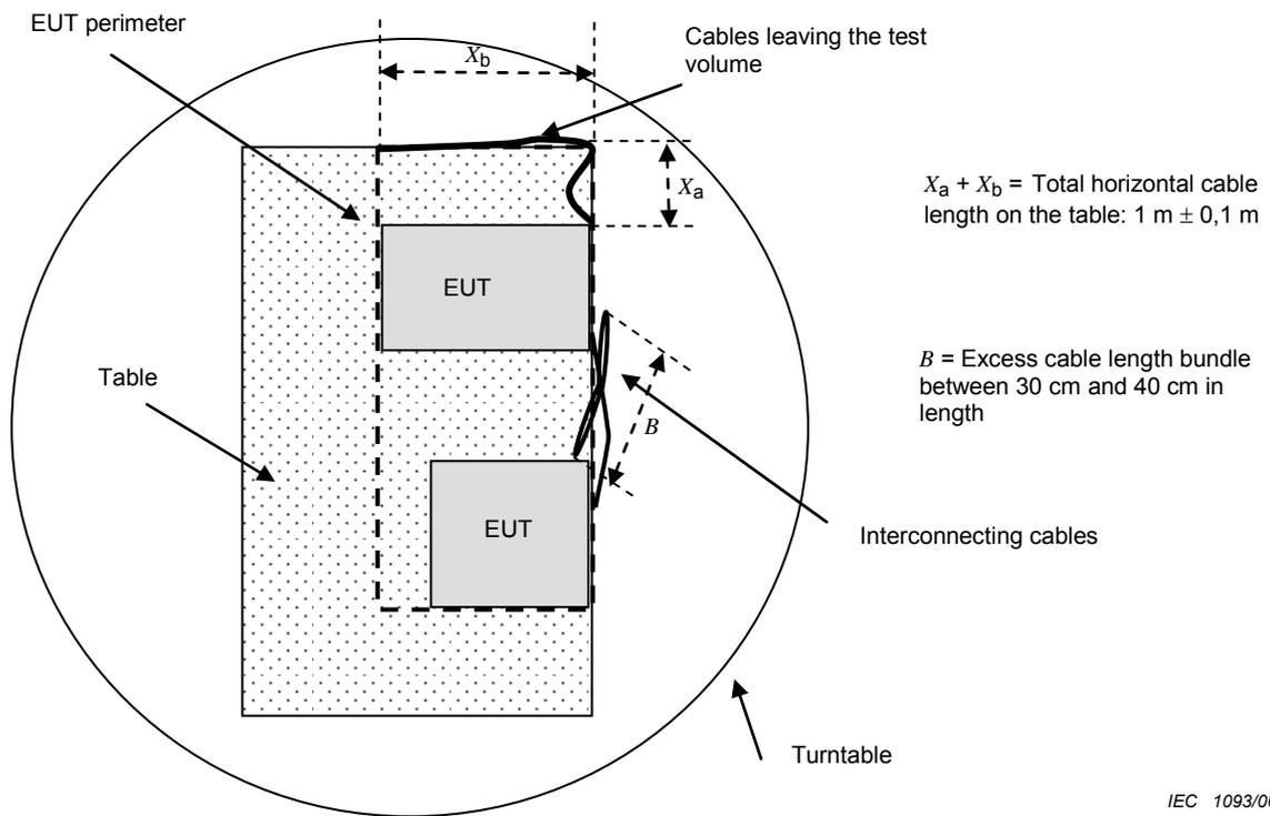
Figure 10 – Test set-up for tabletop equipment – Top view
