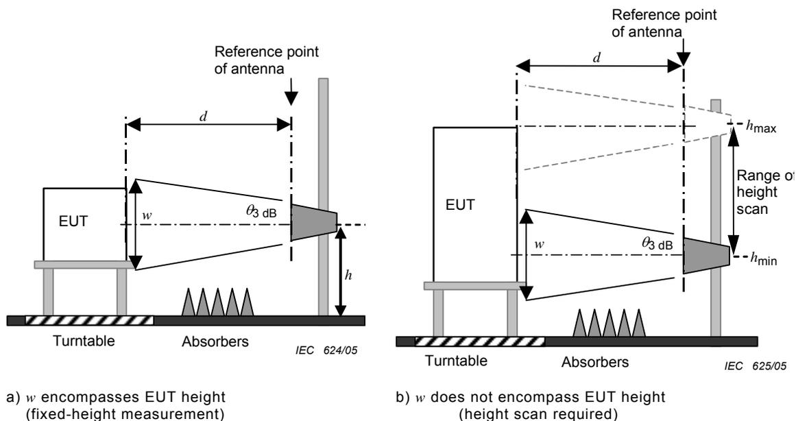
**Figure 15 – Illustration of height scan requirements for two different categories of EUTs**
