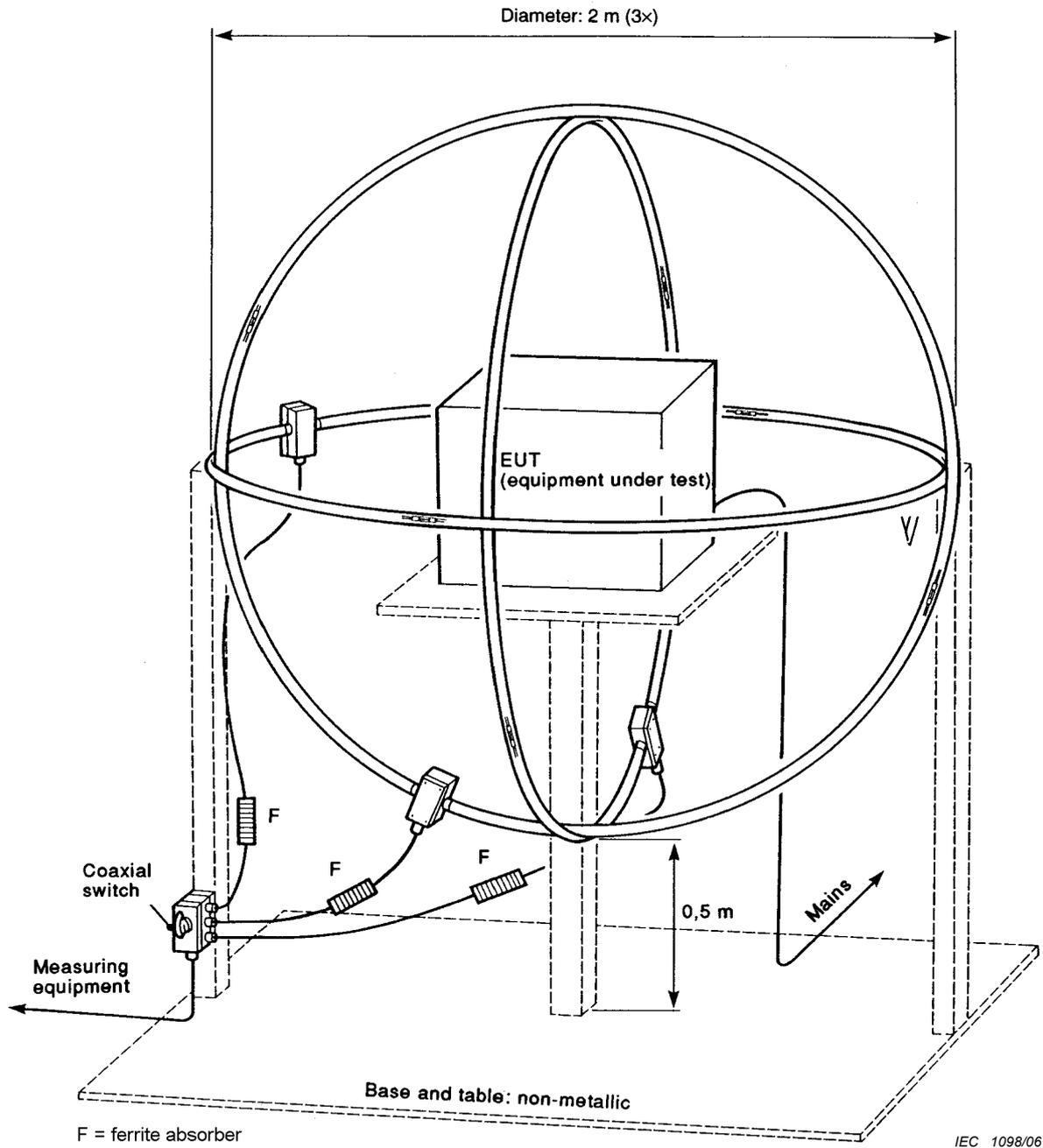
Figure 18 – Concept of magnetic field induced current measurements made with the loop antenna system
