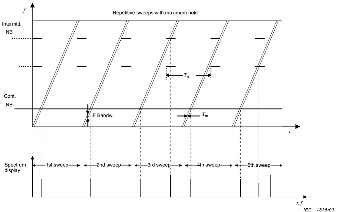
NOTE In the example above, 5 sweeps are required until all spectral components are intercepted. The number of sweeps required or the sweep time may have to be increased, depending on pulse duration and pulse repetition interval.
