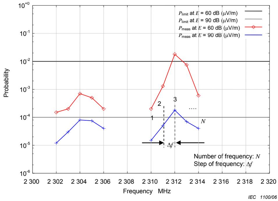
Figure E.2 – Example of APD measurement method 2 for fluctuating disturbances
