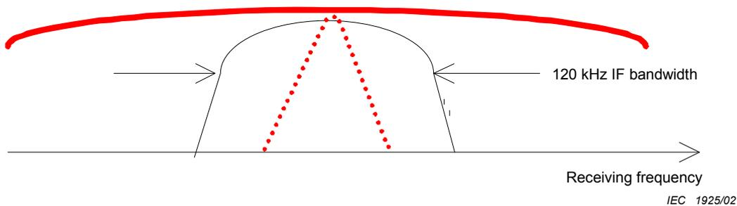
**Figure A.8 – Unmodulated EUT disturbance (dotted line)**
