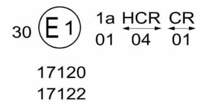
The above example corresponds to the marking of a lens intended to be used in different types of headlamps, namely:
