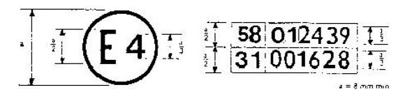
The above approval mark affixed to a vehicle shows that the vehicle type concerned has been approved in the Netherlands (E/4) pursuant to Regulations Nos./58 and  $31./\underline{1}/$  The approval numbers indicate that, at the dates when the respective approvals were given, Regulation No./58 included the 01 series of amendments and Regulation No./31 was still in its original form.
